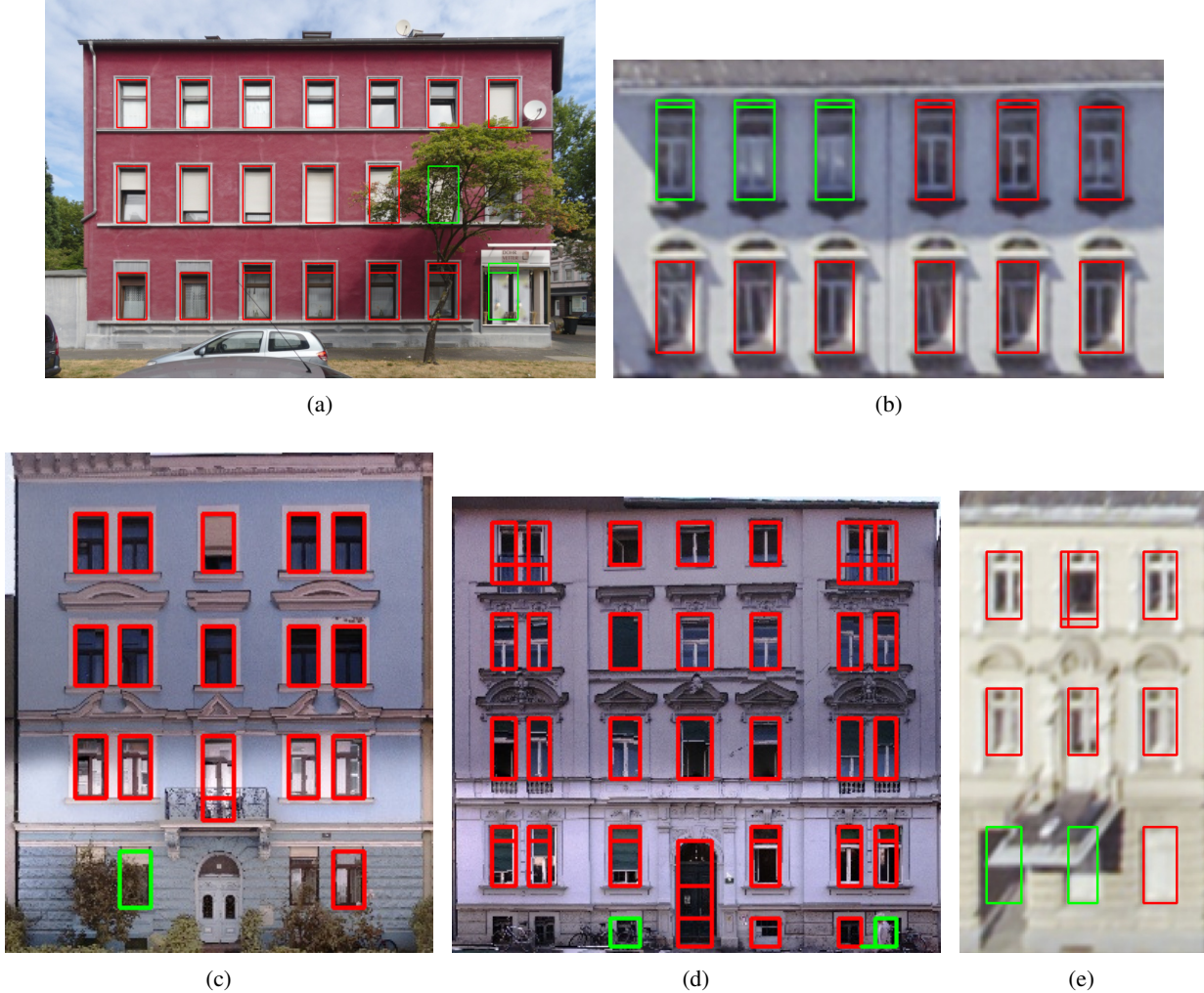
Figure 7: Detection results of the Scaled YOLOv4 network are shown in red. Objects added by the RMD LSTM are annotated with green boxes.
