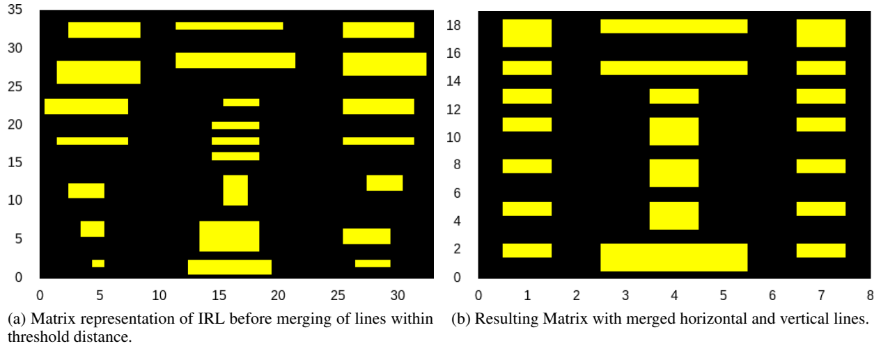
Figure 4: Impact of merging vertical and horizontal lattice lines in the IRL of Figure 3(a). Note that axes are of a different scale, such that the resulting matrix of the simplified IRL is much smaller. [Hensel et al., 2021]
