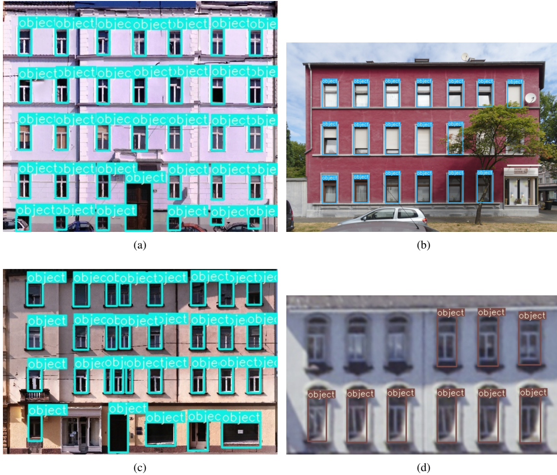
Figure 2: Examples of object detection using Scaled YOLOv4. (a) and (c) are images from the Graz50 dataset [Riemenschneider et al., 2012], (b) has a high resolution whereas the resolution of image (d) is low.
